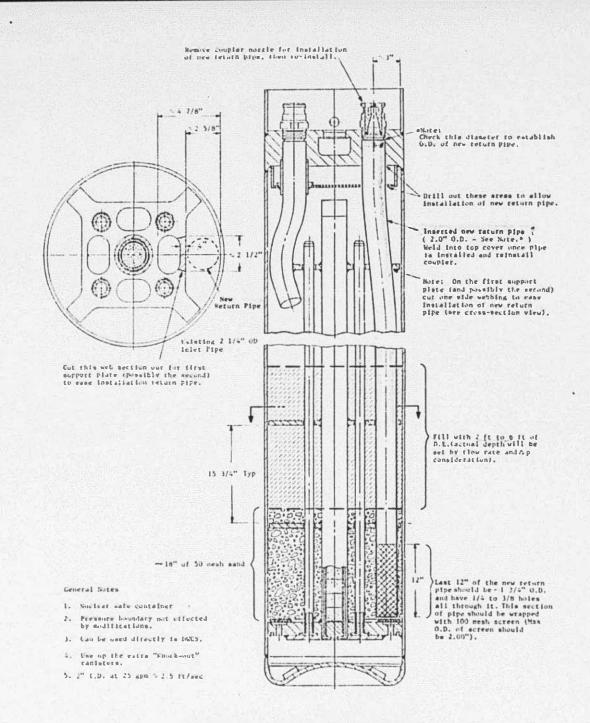
CONCEPTUAL ARRANGEMENT FOR CONVERSION OF "KNOCK-OUT" CANISTER TO A D.E. FILTER WHICH CAN BE USED TO CLEAN UP POOLS & RV
